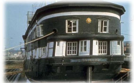
An innovation of Unicorn's designer Sir Robert Seppings, the ship's rounded stern is now the last surviving example left in the world. Not only did this design provide greater strength than a traditional square stern, it gave the ship a greater arc of fire to the rear.
