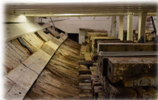
The Hold is the very bottom of the ship and would have been used as a large storage space for food and supplies. With at least 90% of the ship's original timbers intact, the Hold provides a view of the oldest and most unaltered part of Unicorn.
